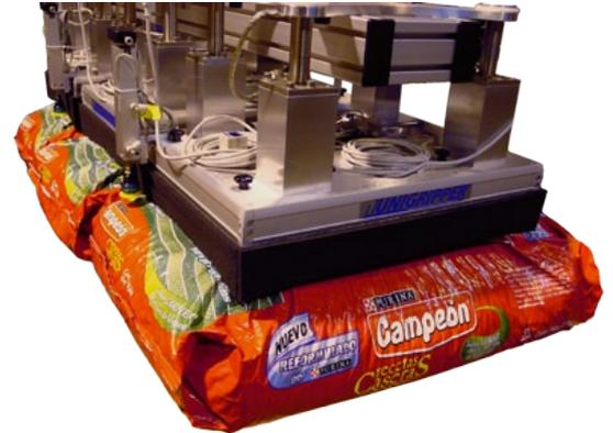
UniGripper with the BagGripper product range has the rare ability to offer one gripper which can handle both palletizing as well as de-palletizing tasks.
