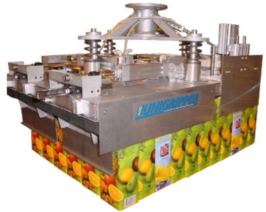
The main spare part for any UniGripper is the foam. Ease of maintenance is granted as the foam is glued on a foam carrier plate, which enables you to change the foam within matters of minutes.
