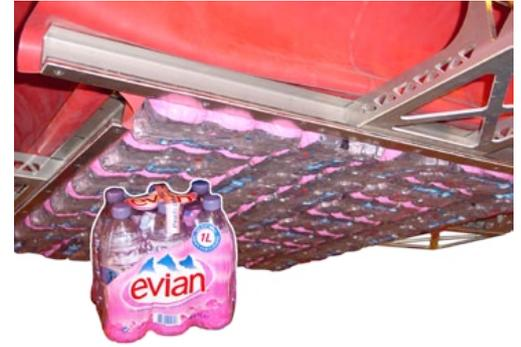
Whether it is one bottle, one row or an entire layer, palletizing or de-palletizing, thanks to the UniGripper solution, the BottleGripper offers the same possibilities as any other of his cousins in the UniGripper product range.
